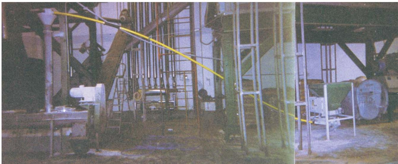
Transport of the product dosaged with the CT-16/360 up to 18 metres length and 6 metres height with optional equipment.
