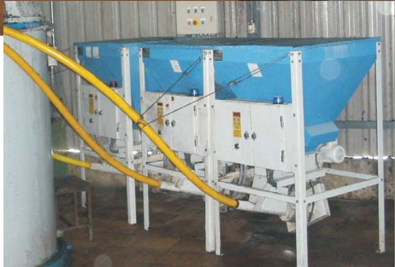
At the end of the conveyor tube the product dose is added continuously and homogeneously in Kg/hour. The mixture is perfect.
