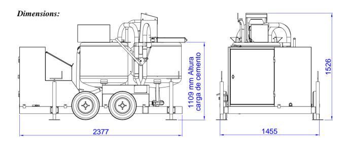
*Machine weight*: 600 Kg (without external elements)
